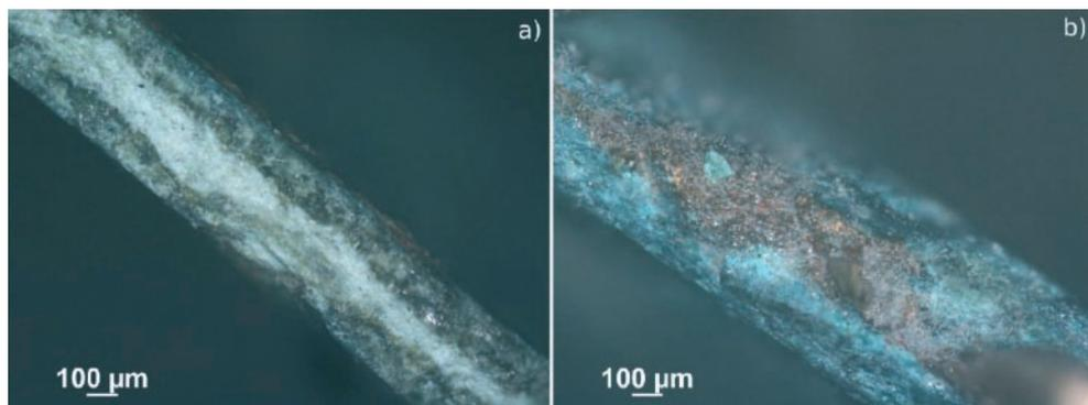
Fig. 2. Dagger from Dargocice. Microscopic image of a cross-section: a – metal phase is invisible; b – part of unoxidised metal is partially preserved in the central area of the cross-section. Photo by B. Miazga
