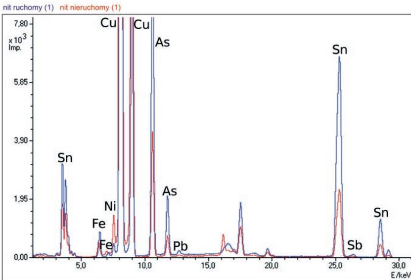
Fig. 8. The ED-XRF spectra of the moveable rivet (blue line) and motionless rivet (red line) which preserved in a dagger
