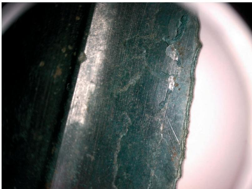
Fig. 5. Scratches and dents visible on the blade of the dagger. Photo by D. Sych
